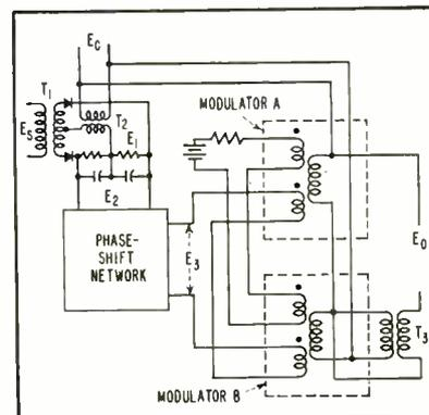
FIG. 1—Two magnetic modulators are used in circuit to maintain input carrier in phase with output carrier
