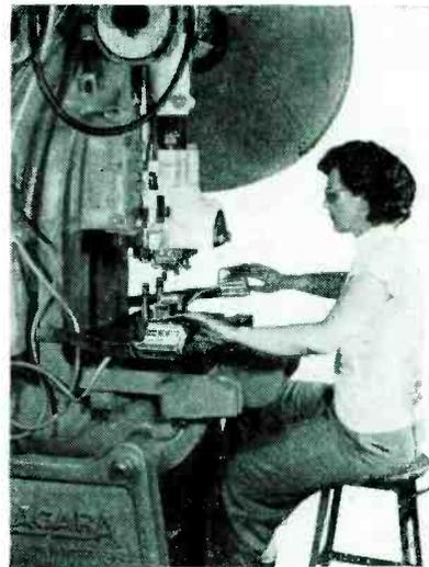
Typical installation of two-hand clutch control on Niagara punch press used in producing electronic components
