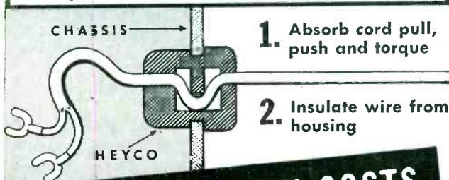
1. Absorb cord pull, push and torque
