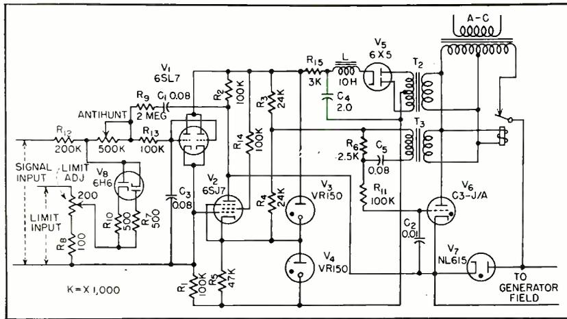
FIG. 4—Generator armature voltage regulator obtains reference voltages from external regulated source. Motor field current control is similar but obtains reference voltage internally
