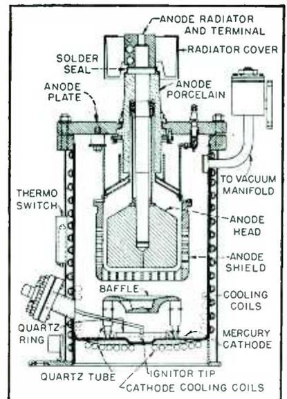
FIG. 1—Cross section of typical pumped-type ignitron
