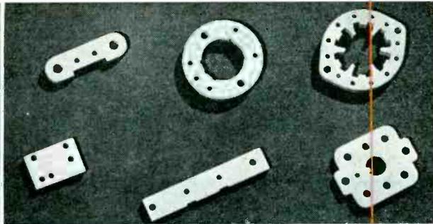
There is no change within the ceramic under extreme conditions of heat and humidity nor any deterioration because of age. Expansion and contraction is practically nil—especially important where close tolerances are factors in assembly. These characteristics of STAR STEATITE are essential high frequency applications where the use of ordinary insulating materials might result in power loss, heating of the insulators and deformation. Write us for samples and complete information.
