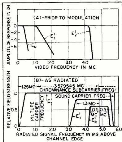
FIG. 8—Bandwidths assigned to luminance and chrominance signals (A) prior to modulation and (B) as radiated. Relative amplitudes of Y, Q and I signals shown are not significant, will vary with picture content
