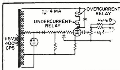
FIG. 8—Circuit of relay-tube amplifier shows fail-safe arrangement with two relays in series with plate
