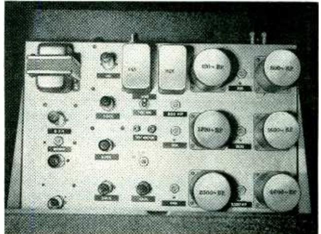
Layout of shielding filters and tubes on analyzer chassis. Screw-driver-adjusted potentiometers equalize insertion losses of filters
