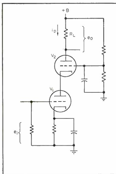
FIG. 1—Basis circuit used as preamplifier for motion-picture iconoscope
