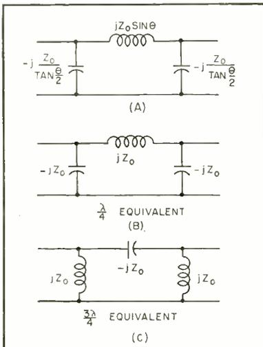
FIG. 1—Pi network equivalent for a lossless line (A) reduces to (B), or to (C) for odd-quarter-wave cases
