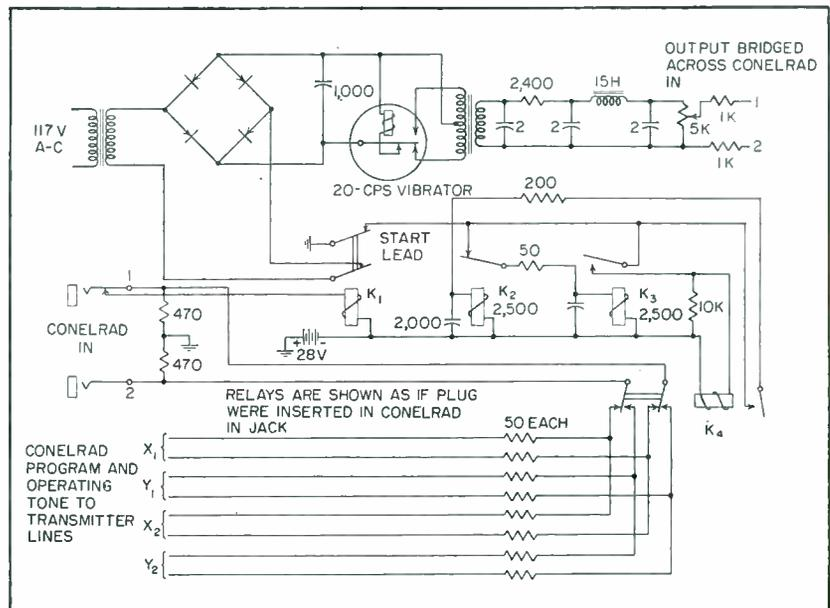
FIG. 1—Complete circuit diagram of the switcher with tone generator, relay time-delay unit and output-line isolating resistors
