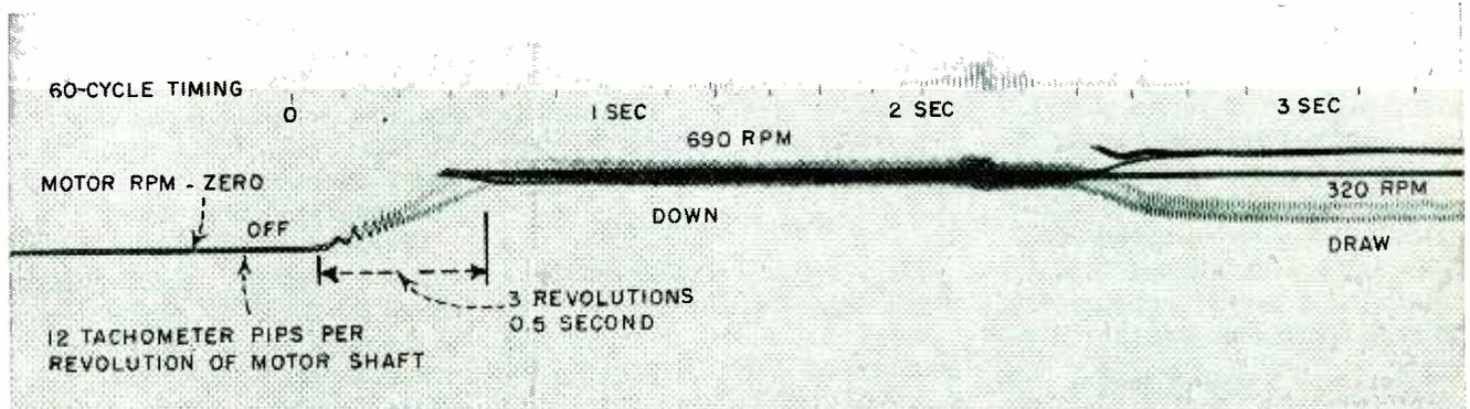
Speed can be changed from zero to 700 rpm in less than three shaft revolutions
