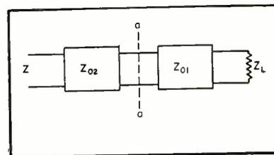
FIG. 3—Tandem network has transformation ratio dependent only on the ratio of the impedances
