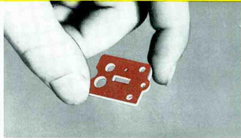
Smooth surface and clean-cut edges show absence of drag, raising, bulging and cracking with NEMA\* test die.
