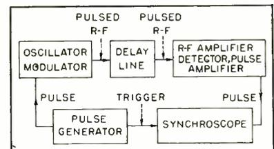
FIG. 1—Method of using delay line as memory, and associated test circuit employing pulse generator and synchroscope
