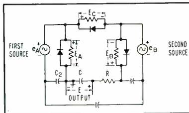
FIG. 3—Phase detector for uhf does not require balanced voltages
