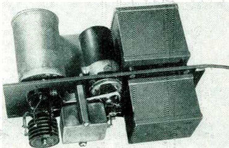
Tone generator produces filtered 20-cps tone to operate transmitter control circuits as program lines are switched. Basic unit is telephone ringing vibrator
