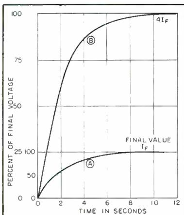
FIG. 2—Time required for field current to reach maximum value, curve A, is reduced by applying overvoltage, curve B, and cutting it off when desired value is reached
