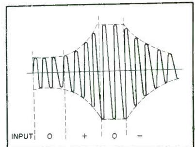
FIG. 2—Response of oscillator output to input signal
