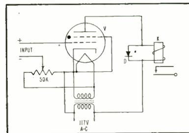
Fig. 1—Circuit of the photocell amplifier
