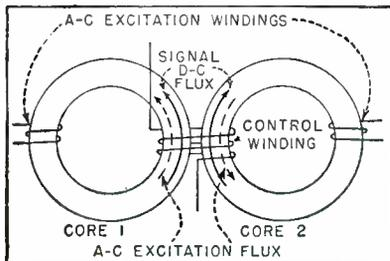
FIG. 1—Signal on d-c control winding of magnetic converter will aid the excitation flux in one core while opposing the flux in the other
