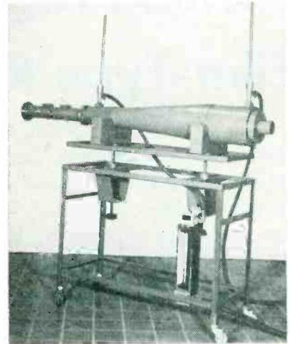
Water load for uhf. Flowmeter is located under table
