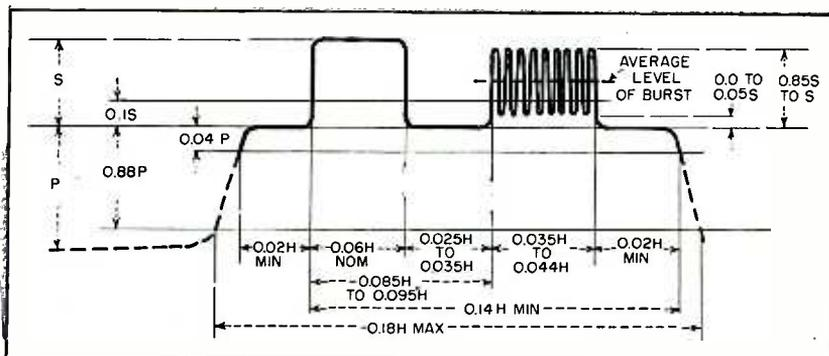
FIG. 4—Early form of color synchronizing burst, having average value above blanking. Compatibility difficulties resulted in revision of this waveform to final form shown in (5) of Fig. 1
