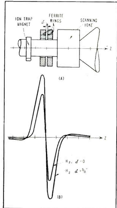
FIG. 2—Ceramic focusing unit (A) uses two ceramic rings to obtain field intensity plot (B)
