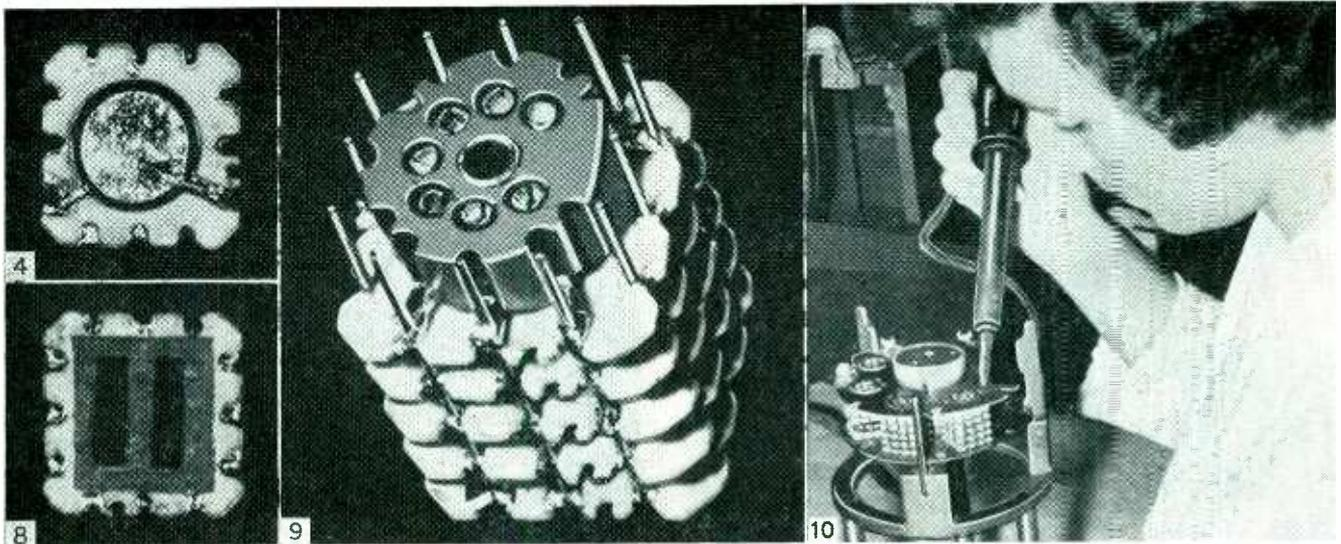
Wafers, modules, mechanized production line and (at right) the final submarine detector unit. Numbers on diagram correspond to numbers shown on photos above
