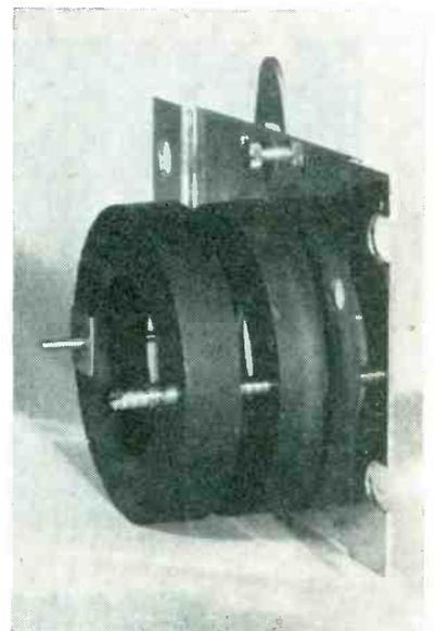
Screw adjustments on ceramic focusing unit permit adjustment of focus by changing spacing between magnets
