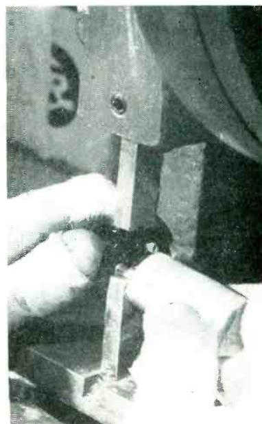
Method of crimping capacitor lead to pin of octal base
