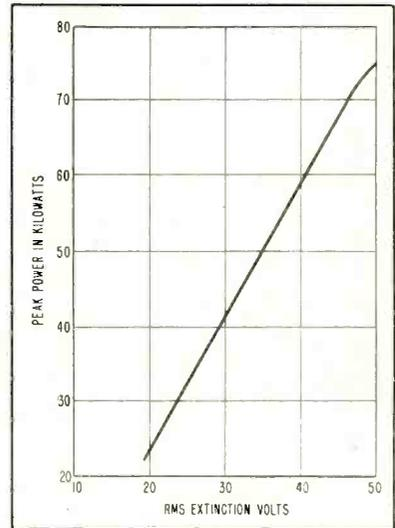
FIG. 2—Plot of power against extinction voltage of NE-2 bulb shows good linearity
