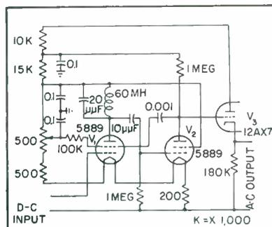
FIG. 3—Circuit of oscillator converter
