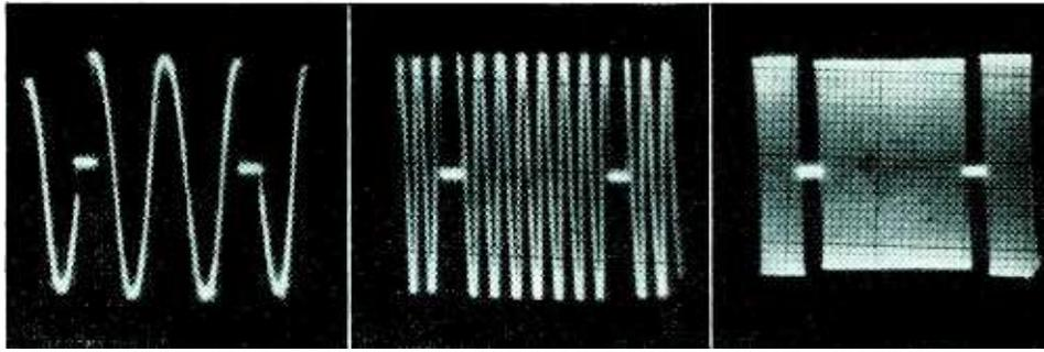
Vibrator output terminal 1 (Fig. 2) with 200 cps, 1 kc and 25 kc, respectively fed to inputs. The 25-kc input signals are unequal by 4 percent
