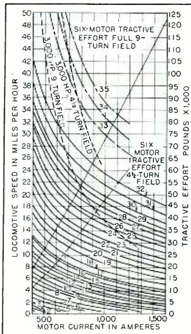
FIG. 2—Performance curves of ignitron locomotive. Speed for a given motor current is indicated by solid curves
