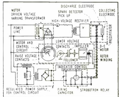
**FIG. 1—Sparking rate of electrical precipitator is electronically controlled**
