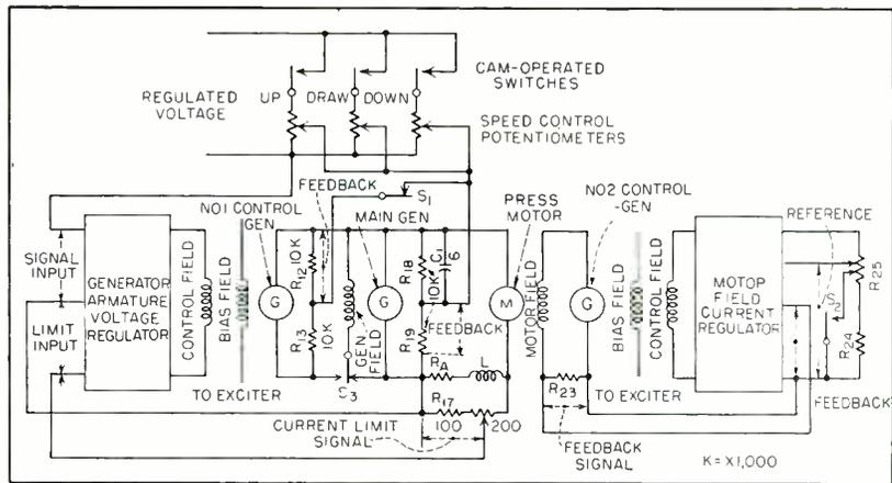
FIG. 3—Draw-press drive uses two regulator units to control generator armature voltage and motor field current. Cam-operated switches select proper reference voltage for different portions of press cycle
