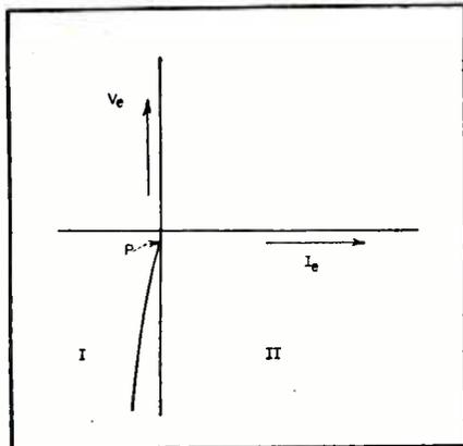
FIG. 3—Emitter characteristic curve in region I before any switching action takes place
