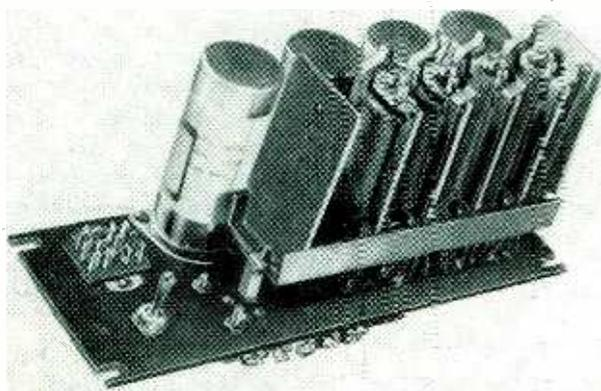
Time-delay switcher transfers audio program and control tone from one set of lines to other every 30 seconds. Large capacitors across relay coils provide delay
