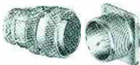
**AN** Designed to Air Force—Bureau of Aeronautics—requirements. Now widely used for all instruments requiring electrical circuits. Coupling nut connection and disconnection. Two plug types; 3 receptacles with variations and clamp accessories, in 15 shell sizes and more than 250 insert arrangements. A type for every need. Ask for "AN" Bulletin.
