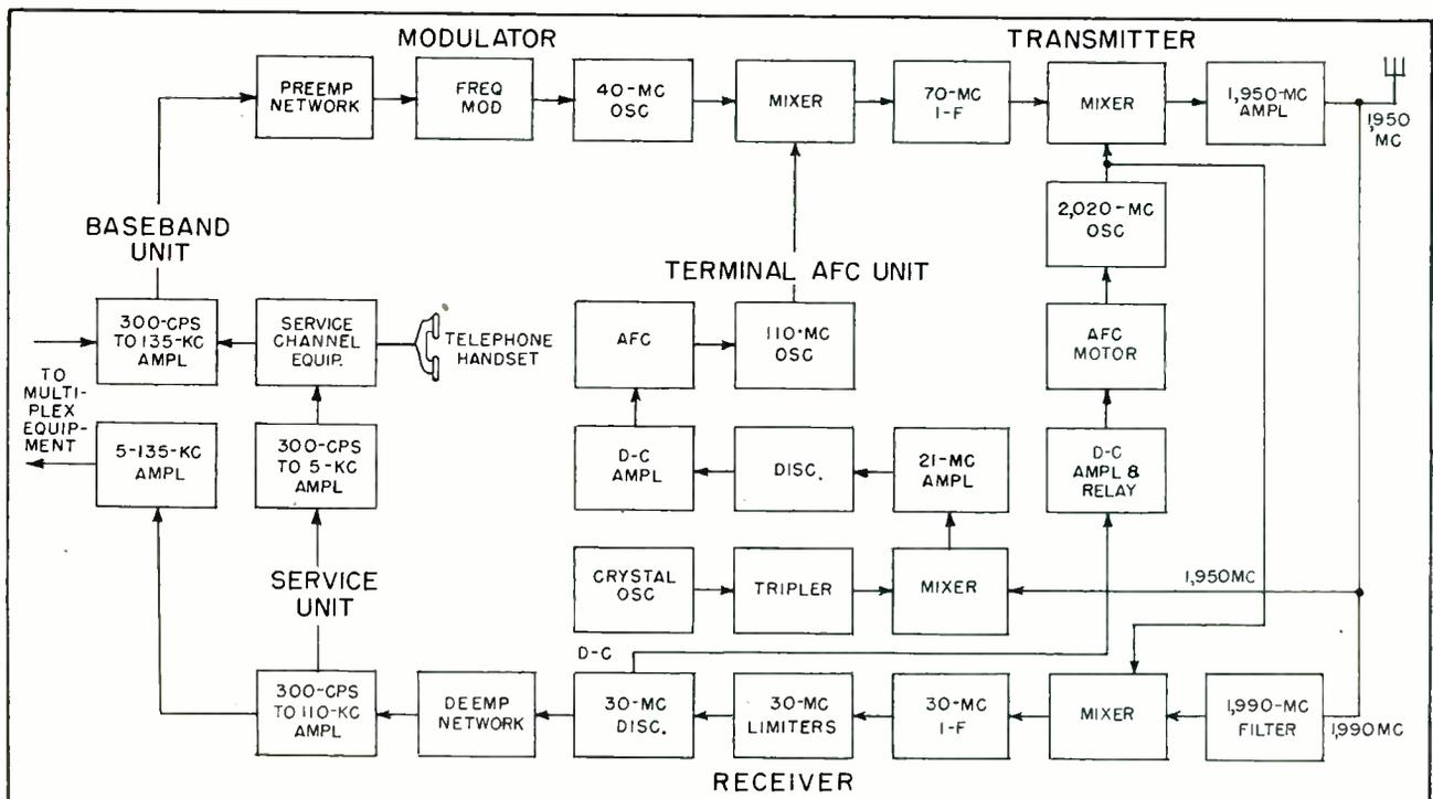
FIG. 1—Terminal station comprises transmitter, receiver-modulator, afc unit, baseband amplifiers and service-channel equipment
