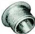
**GS (AN)** Designed for applications demanding hermetic sealing under high pressures in a temperature range from minus 300F to plus 600F. 2 basic shell designs. NEF threaded coupling nut. Steel shells and steel contacts. Mate with AN Series. See "AN" Bulletin or "GS" Bulletin.
