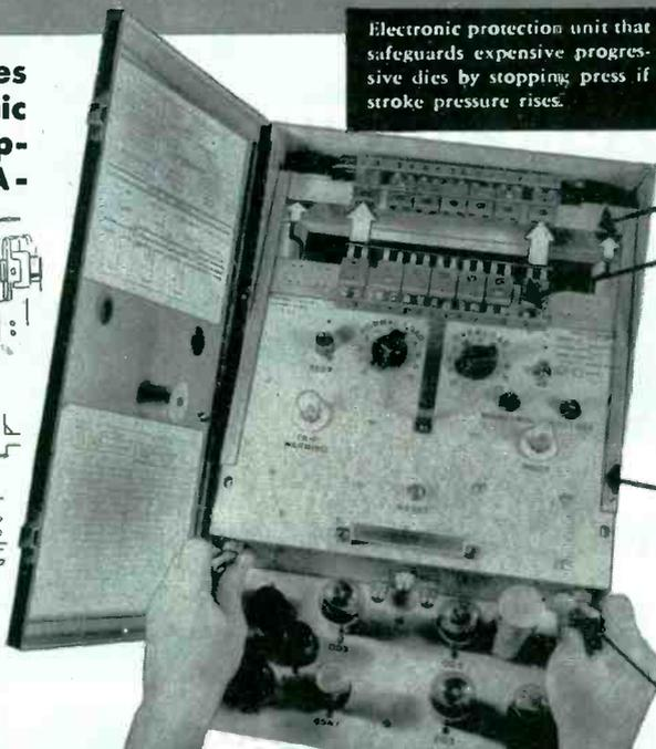
Electronic protection unit that safeguards expensive progressive dies by stopping press if stroke pressure rises.
