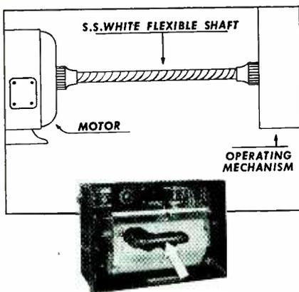
The short coupling shaft that was used provided a positive, vibrationless linkage which eliminated the need for aligning the connected spindles. This not only assured better operation, but it also simplified assembly and reduced production time and costs. It will pay you to consider S.S. White flexible shafts whenever you have to transmit rotary power between two points. They're economical and dependable and often make possible substantial savings in manufacturing and assembly costs.
