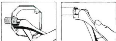
Examples of two uses for roller-jaw pliers. At left, pliers serve for tightening locknut in outlet box. At right, they are being used to remove burrs from metal tubing after sawing
