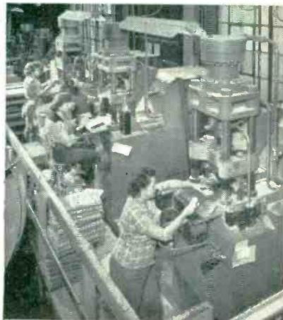
Production operations—including mixing, molding, drilling, tapping and stamping are mechanized. This assures uniform quality, fast operation, low costs.
