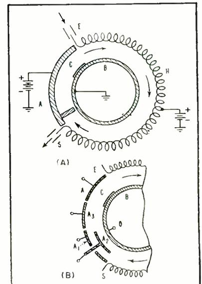
FIG. 5—Circular traveling-wave tube (A) and improved version (B)
