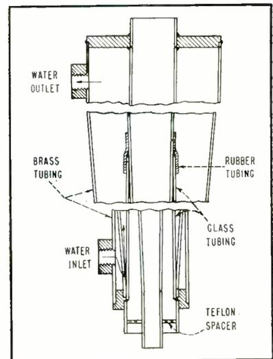
FIG. 1 — Cross-section of high-power water load
