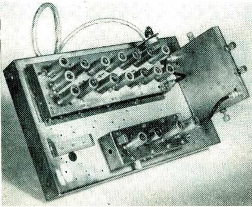
Complete memory device, with quartz slab in its holder at right on chassis
