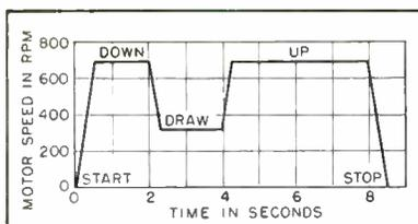
FIG. 1—Range of motor speeds required during one press cycle
