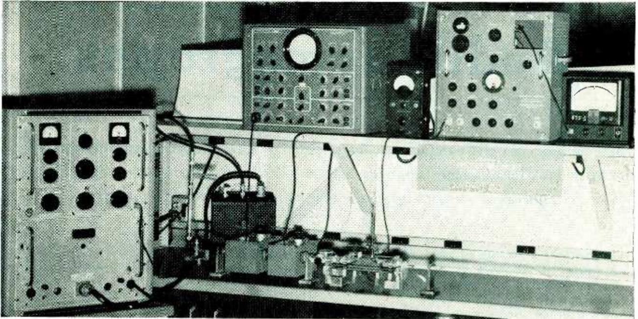
Millidecibel test setup. Equipment on shelf includes: monitor scope, agc voltmeter, amplifier and indicator. Lower deck holds: power supply, signal source, tuner and directional coupler, buffer attenuator, two cavity wavemeters, precision attenuator and slotted line and test sample. Variable short is not shown
