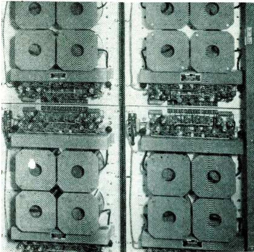
Partial view of four-tube rack assemblies showing shields over tube faces. There are three four-tube units in each rack for the SEAC computer at National Bureau of Standards in Washington, D. C.
