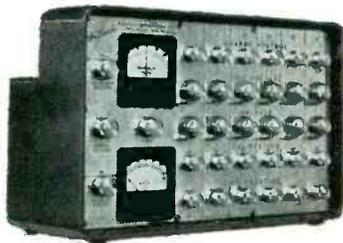
**Model 82-6 Bridge Balance and Strain Indicator Unit**
