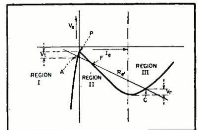
FIG. 7—Emitter characteristic in regions I, II and III. The emitter current and voltage vary along the N-shaped line indicated, with stable points at A and C
