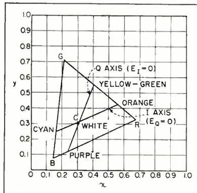
FIG. 7—The I and Q axes, showing colors reproduced when only one chrominance component is active. The color triangle RGB bounds color gamut covered by proposed NTSC primary colors (item III-D-1)
