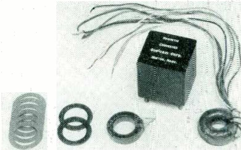
Built-up cores of magnetic converter are wrapped with excitation and control windings and the entire unit is mounted in a box about  $1\frac{1}{2}$  in. square
