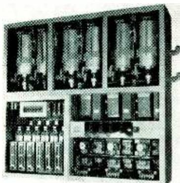
Locomotive ignitron cubicle houses six tubes and associated apparatus
