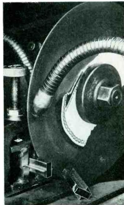
Method of cutting roll-formed waveguide to length with abrasive cut-off disk on shaft of power saw
