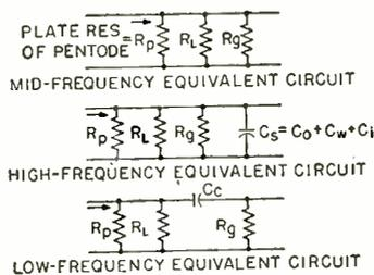
FIG. 1—Basic circuit, characteristic response curve and equivalent regions for three different regions of the audio spectrum
