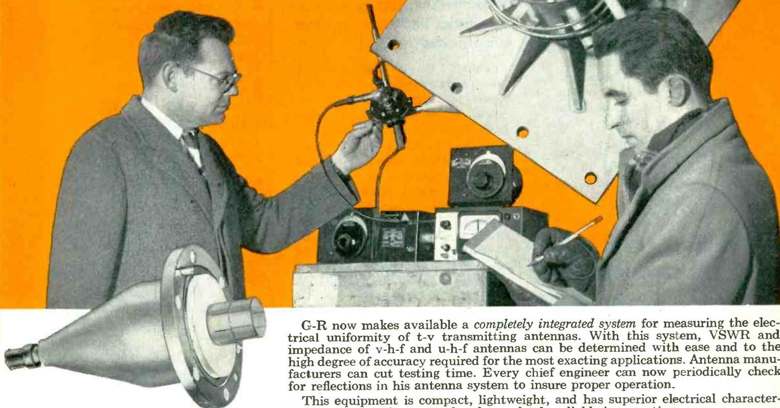
G-R now makes available a *completely integrated system* for measuring the electrical uniformity of t-v transmitting antennas. With this system, VSWR and impedance of v-h-f and u-h-f antennas can be determined with ease and to the high degree of accuracy required for the most exacting applications. Antenna manufacturers can cut testing time. Every chief engineer can now periodically check for reflections in his antenna system to insure proper operation.
