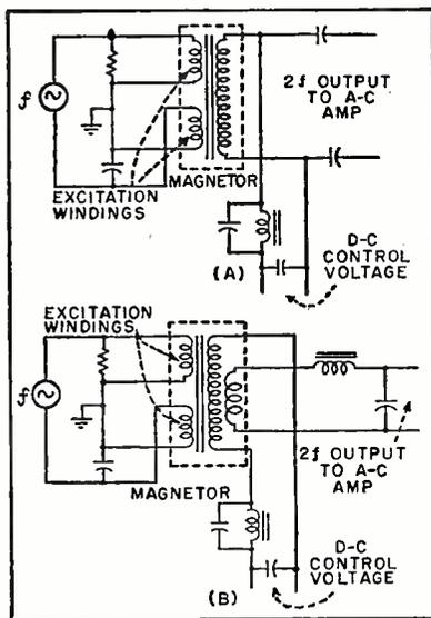
FIG. 4—Methods used for filtering fundamental from output of second-harmonic converter. Converter (B) has a separate secondary for output
