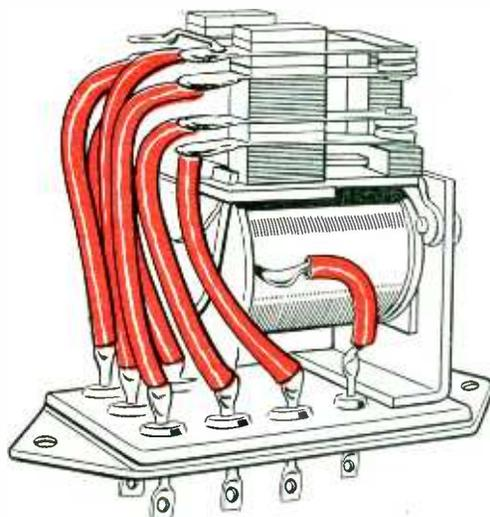
A Price Electric Corporation, Frederick, Maryland relay, series G000HS, shown at actual size, without its protective cover. Illustrated in red is BH "1151" used to insulate connecting leads, shunts and pigtails.
