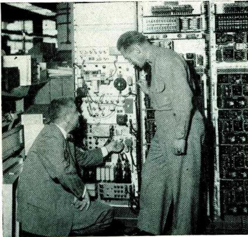
Terminal-station equipment. Rack at left contains microwave transmitter receiver, modulator and a/c circuits; multiplex equipment occupies remaining racks
