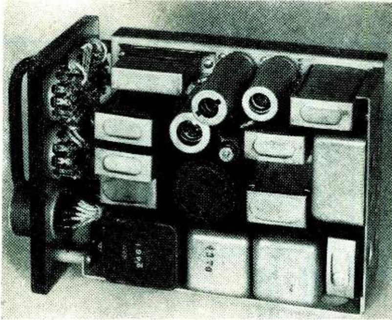
Top chassis view shows little space has been wasted in automatic pilot monitor. Fail-safe circuits monitor the monitor's activities
