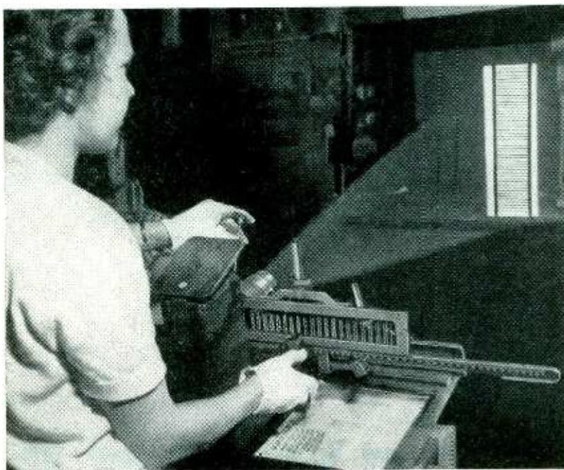
Modified slide projector throws ten-times enlargement of tube grid on screen as shown, during 100-percent inspection for pushed, spread or damaged turns. Right hand is on knob of rack-and-gear arrangement for moving grid carrying frame through projector. Left hand is on rod used for mangling defective grids
