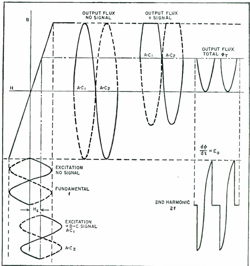
FIG. 2—Second-harmonic signal is produced in magnetic converter by displacement of the axis of symmetry by the d-c signal
