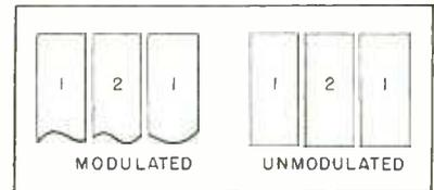
FIG. 3—Modulation on input (left) results in distortion, whereas clean signals (right) allow easy comparison
