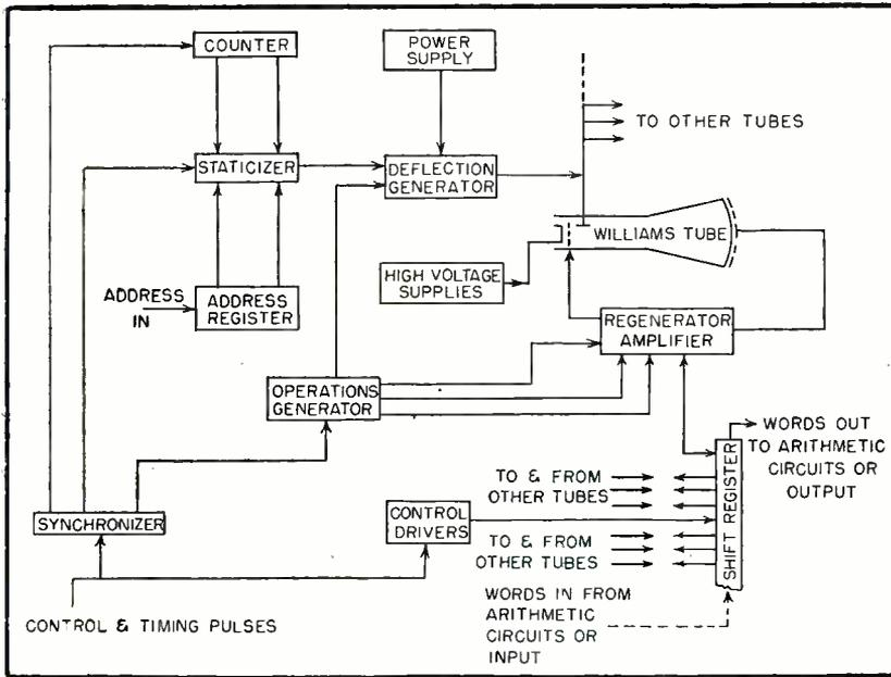
FIG. 5—Block diagram of electrostatic memory system using modified conventional cathode-ray tube
