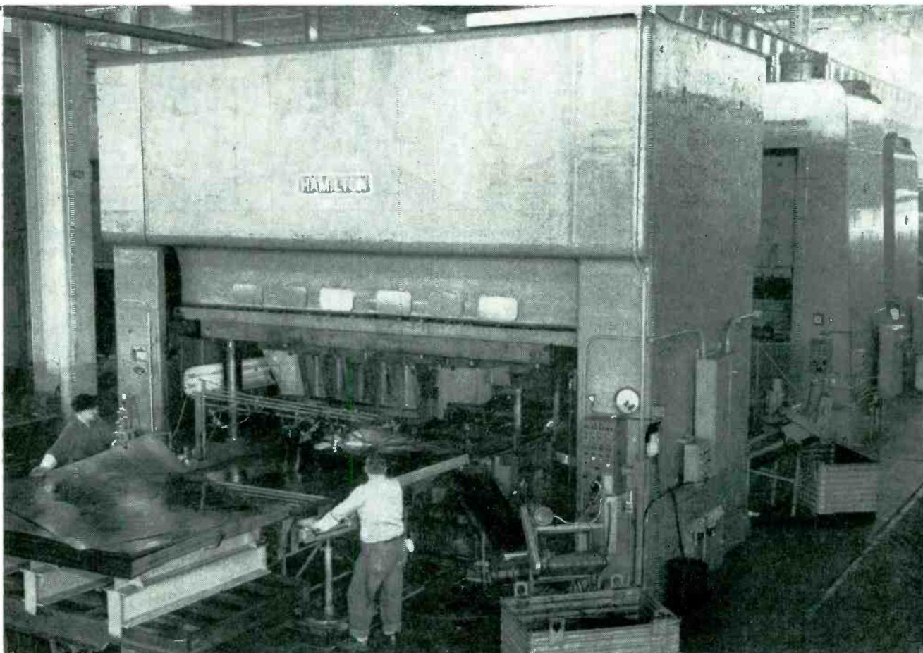
Output of thousand-ton press has been increased 25 percent by installation of electronic drive-motor controls
