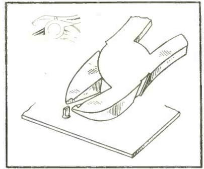
Closeup views of pliers, showing combination cutting and crimping jaws and shape of crimped terminal
