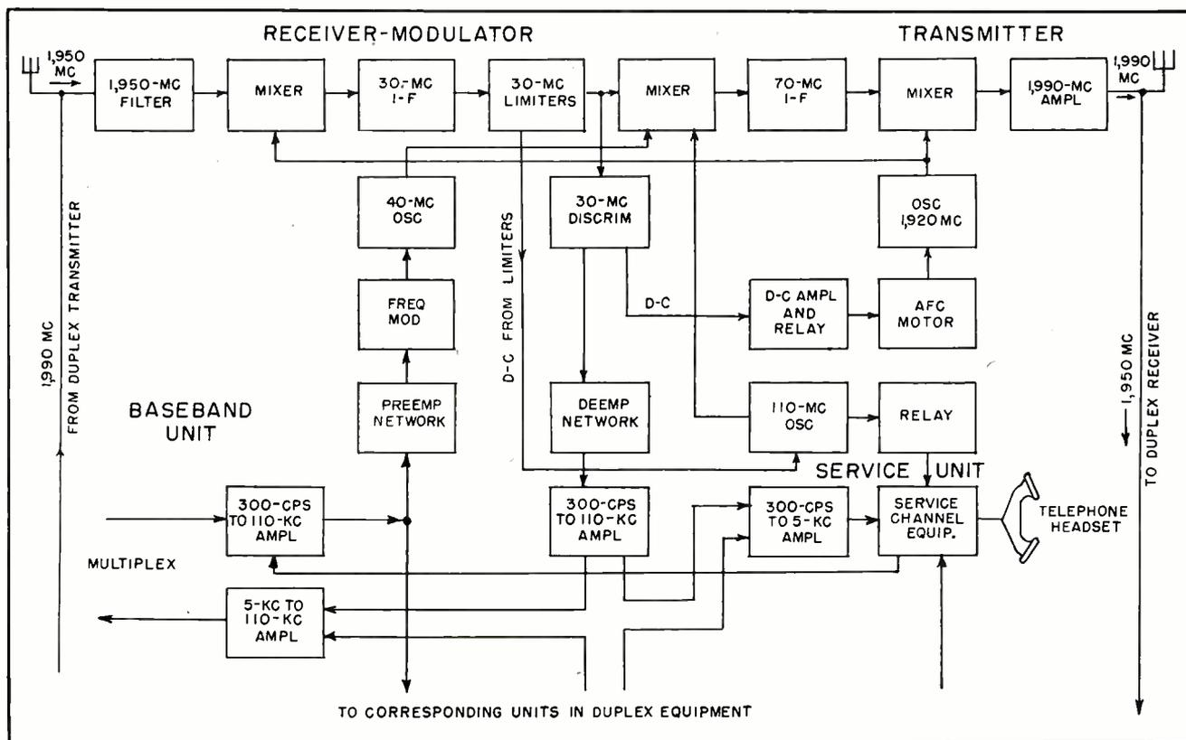
FIG. 2—Repeater stations have duplex transmitters and receiver-modulator units. Baseband amplifiers, service-channel equipment and multiplex gear are shared
