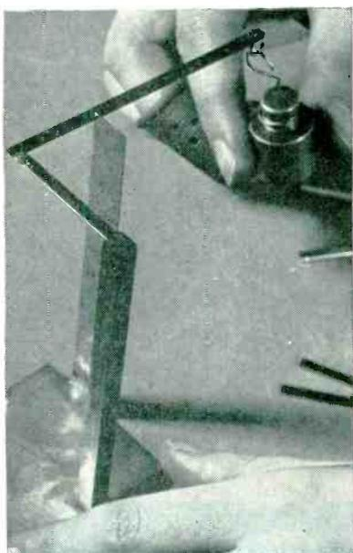
Twisting cathode sleeve to check strength of lock seam
