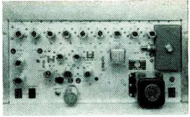
Receiver-modulator chassis 2C3I local oscillator is housed in shielded compartment at right
