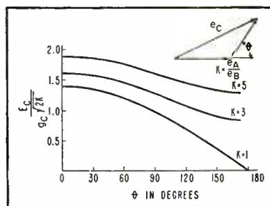
FIG. 4—Characteristics of phase detector described in text
