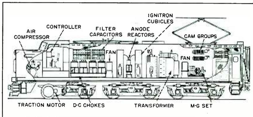
Artist's drawing of electric locomotive shows position and relative size of ignitron cubicles located in center of cab
