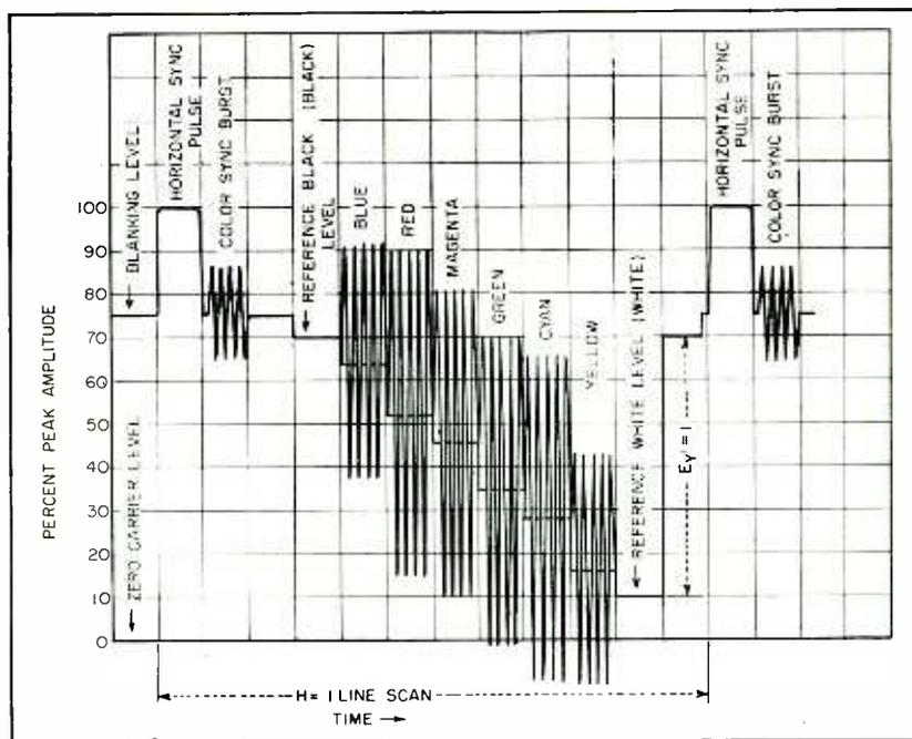
FIG. 3—Video modulation waveform resulting from scanning a single line of a bar chart containing fully saturated primary and complementary colors. The dashed line (average of chrominance oscillations) represents corresponding luminance levels. Burst and chrominance frequencies not drawn to time scale
