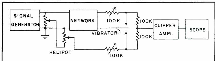
FIG. 1—Block form of the signal comparator
