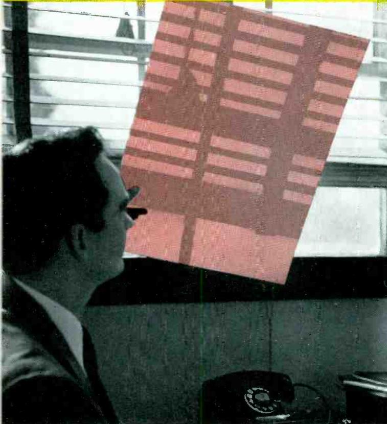
Sheet uniformity, directly related to punching quality, is demonstrated by the clear translucency of this material.
