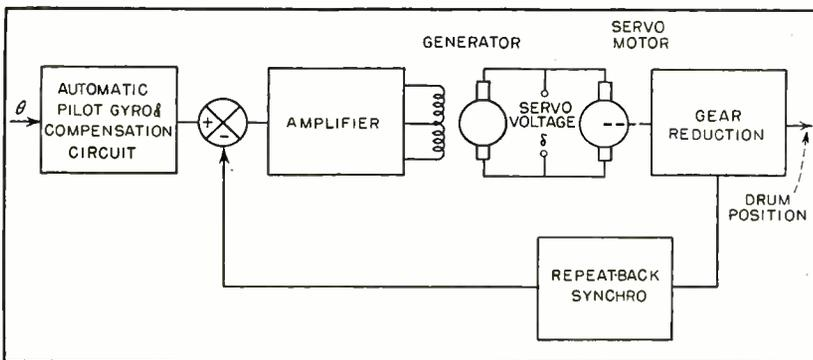
FIG. 4—Simplified diagram of automatic pilot servo system
