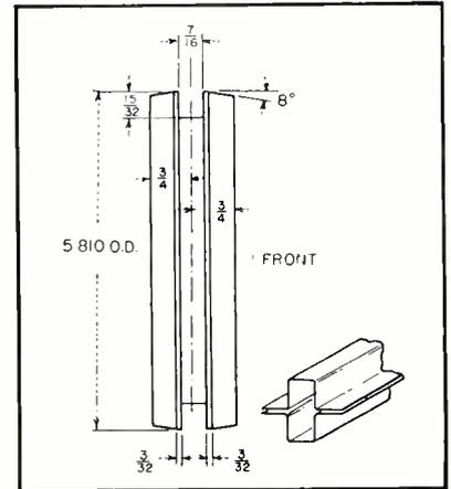
Electrode wheels used for double-seam welding of waveguides, and sketch showing shape of finished waveguide
