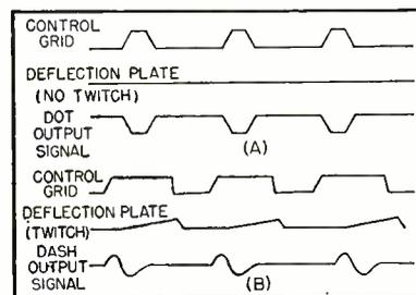
FIG. 3—Waveforms for observing dot signal (A) and dash output (B)
