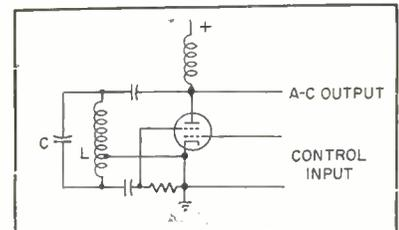
FIG. 1—Basic oscillator circuit for d-c conversion
