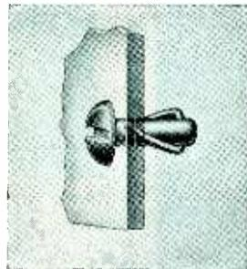
**SPRING-LOCK** One-piece fastener for blind holes has load-carrying steel spring wire. Spring steel arms lock fastener securely, prevent loosening under vibration. SPRING-LOCK will work with varying panel thicknesses, locks with a twist of the wrist. SPRING-LOCK is now available in high-impact plastic. The molded design permits heads to be made in various shapes for refrigerator shelf supports, washer knobs, brackets. Available in a wide variety of shapes and sizes, and also in custom designs.
