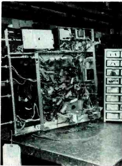
Method of using chassis turntable at repair position alongside assembly line for dip-soldered television receivers at G-E plant in Electronics Park, Syracuse. Edges of table are covered with tempered Presswood, same as on top
