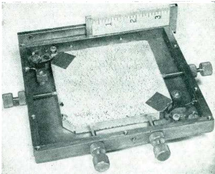
Fused-quartz slab mounted in holder for use as 400-microsecond solid ultrasonic delay-line memory, with cover removed. Inexpensive commercial-quality material can be used, as internal strains and small bubbles do not produce any spurious signals greater than 60 db down from the main received signal. Projecting knurled adjusting screws permit shifting position of quartz slab to get desired folded-path configuration and hence desired delay
