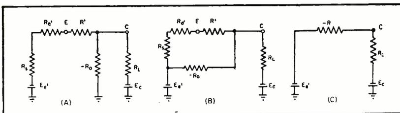
FIG. 6—Equivalent circuit in region II as seen by the load
