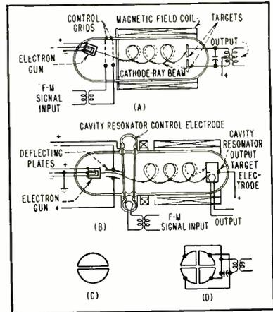
FIG. 2—Cathode-ray oscillator in two forms (A) and (B) uses two different target electrodes (C) for frequency doubling (D)
