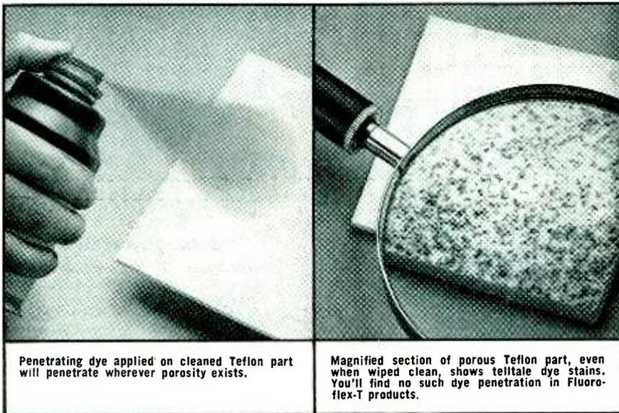
Penetrating dye applied on cleaned Teflon part will penetrate wherever porosity exists.
