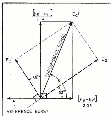
FIG. 5—Phasor diagram showing relative phase angles of color burst and chrominance components (item III-D-1)
