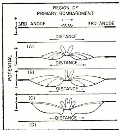
FIG. 2—Potential diagrams show distribution across tube face. Successive steps in charging of screen when beam is turned on a single spot
