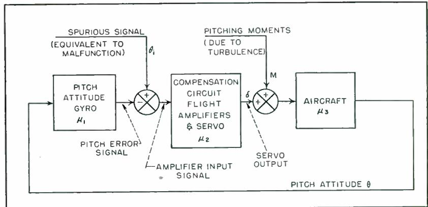
FIG. 1—Simplified block diagram of aircraft under automatic pilot control
