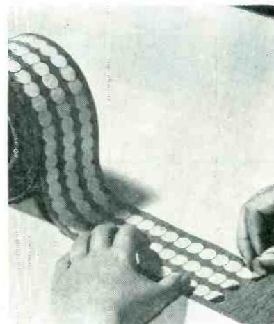
Method of removing masking disc from crepe paper liner
