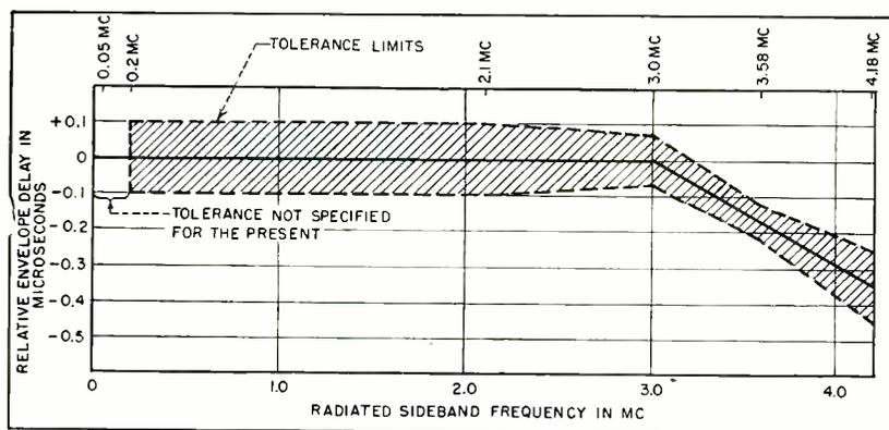
FIG. 6—Transmitter time delay specification which compensates for phase characteristic of average receiver (item III-B)
