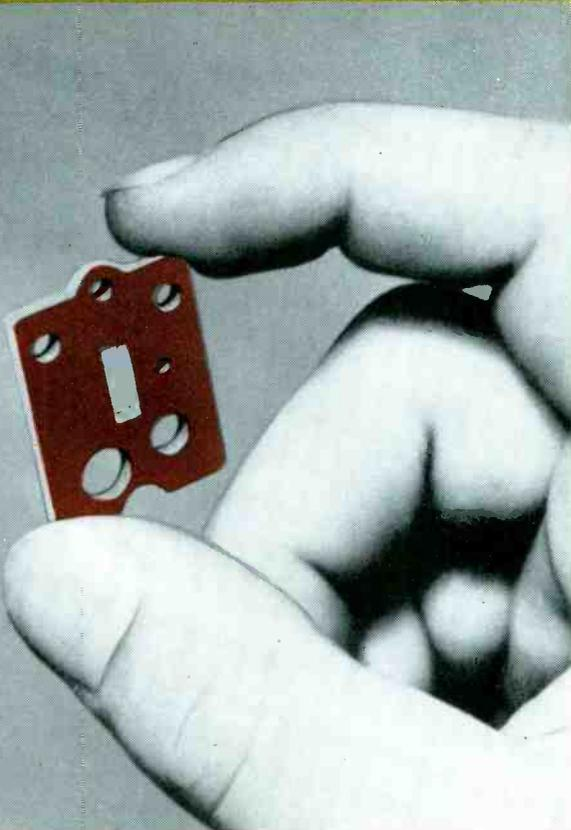
*Cold-punching from NEMA\* test die—holes are clean-cut, surface is smooth, edges show no chipping.*
