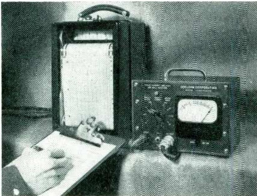
The d-c amplifier and null indicator using magnetic converter has low and high impedance outputs for recorder or control-system use. Direct-reading meter will respond to signals as low as  $1 \mu\text{v}$  at  $0.002 \mu\text{a}$
