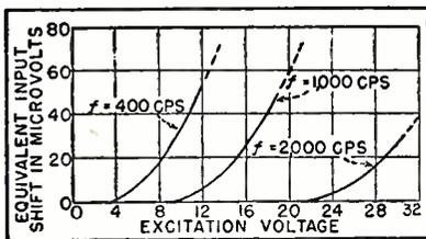
FIG. 3—Shift in zero caused by variation of excitation voltage in second-harmonic magnetic converter
