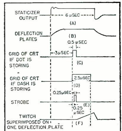
FIG. 6—Timing of the memory cycle is explained in text
