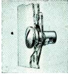
**QUICK-LOCK** For fastening removable access doors and panels. Because of its ease of installation, QUICK-LOCK is ideal for assembling removable panels. A 90° turn locks it in place. Stud is self-ejecting when unlocked; visual inspection shows whether fastener is locked. Spring loading takes initial load; solid supports carry increased load. Available in a wide range of sizes.
