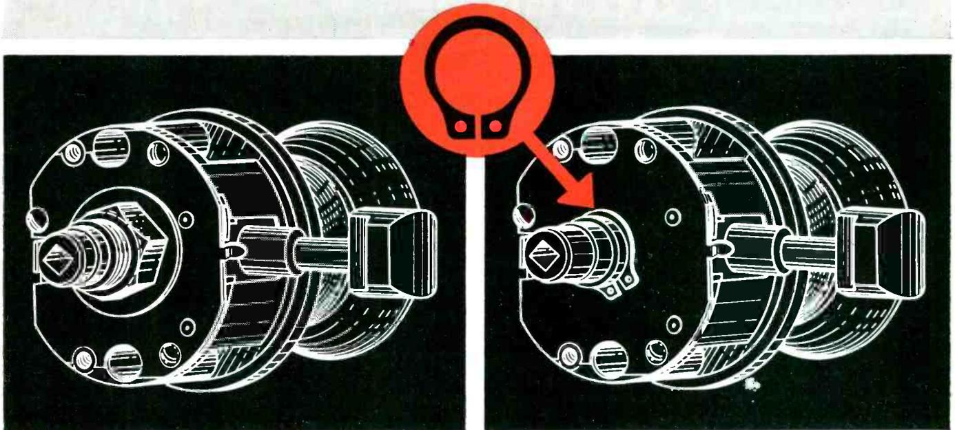
**OLD WAY.** Main shaft required costly threading. Assembly was slowed by the double application of washer and nut and time-consuming tightening operation.
