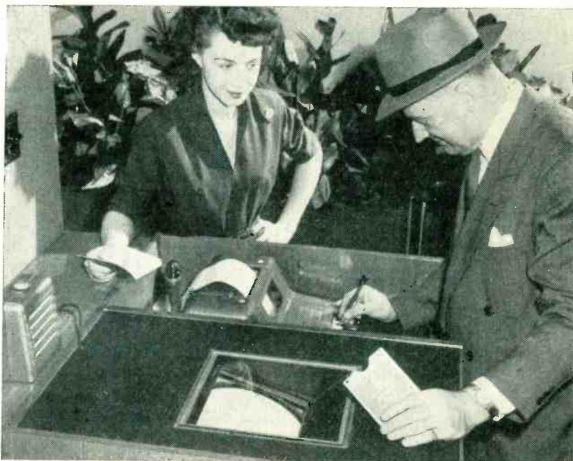
**SIGNATURE** of branch depositor is recorded in bank's main office by wired autograph system. Tv and intercom give access to main office records as . . .
