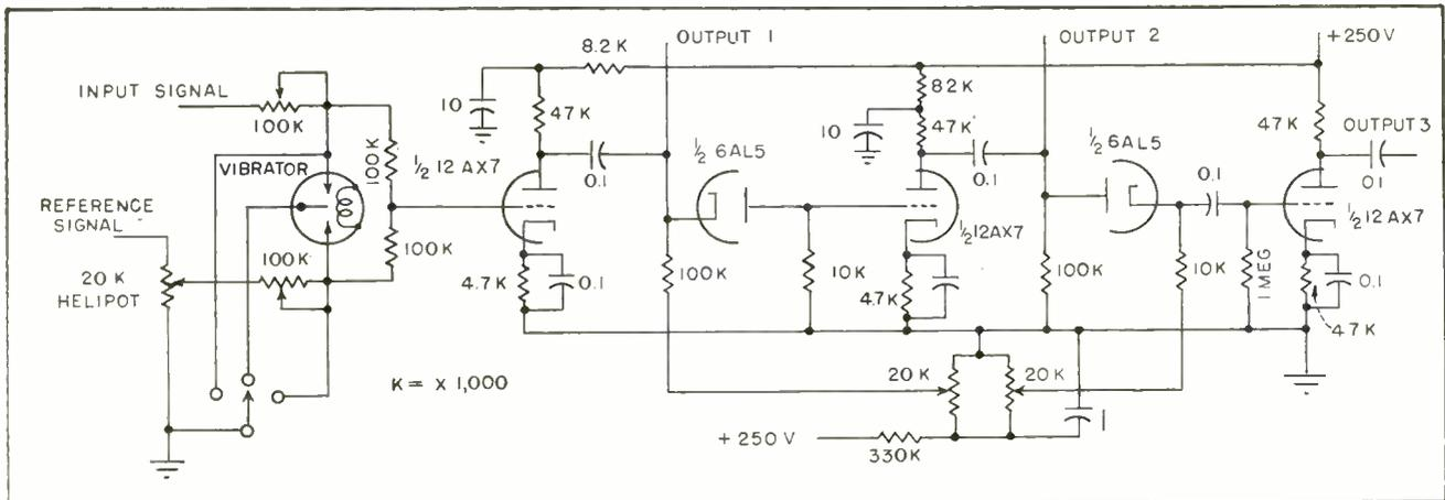
FIG. 2—Fundamental circuit of the clipper-amplifier comparator that can be used with either d-c or a-c inputs
