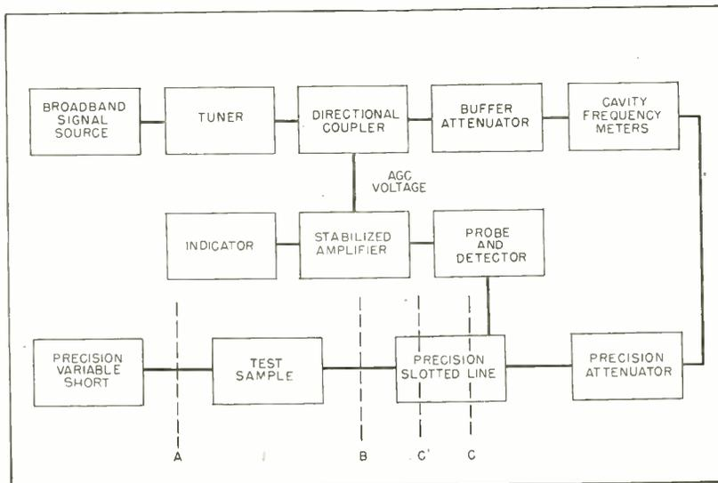
FIG. 1—Equipment setup for millidecibel attenuation measurements
