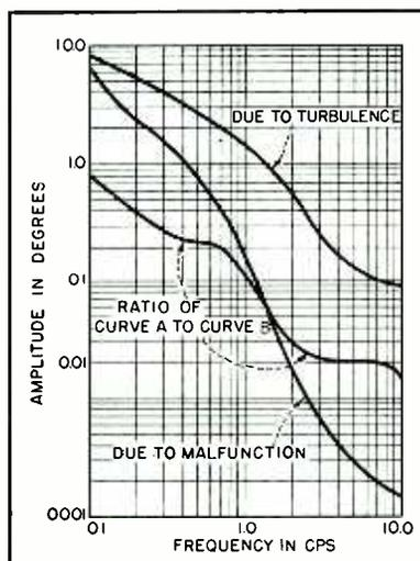
FIG. 7—Allowable aircraft motion before cutoff. From top to bottom (at 10 cps) curves are B, C and A
