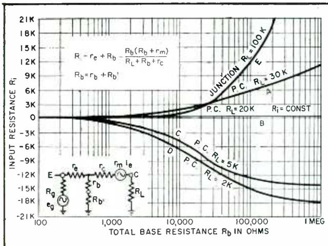
FIG. 1—Variation of input resistance of the grounded-base transistor with total base resistance
