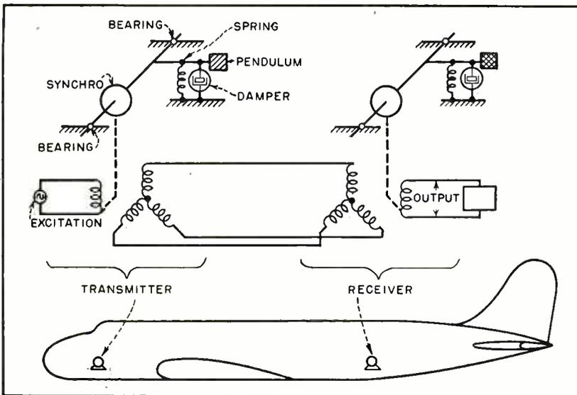
FIG. 3—Schematic diagram of angular accelerometer arrangement
