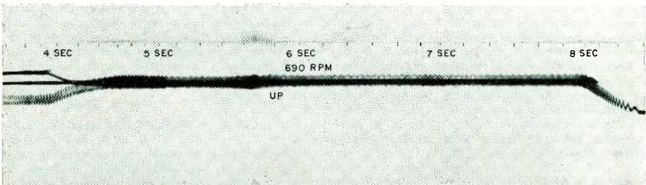
FIG. 5—Oscillogram of complete press cycle, showing rapid speed changes made possible by use of thyatron regulator system
