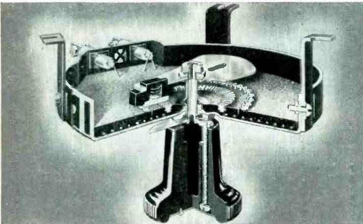
**CUTAWAY VIEW OF TYPICAL WARD LEONARD RHEOSTAT.** Eastman Kodak's Recordak engineers chose a 13-in. Vitrohm rheostat to control lamp voltage in the Recordak Micro-File machine. It provides 161 graduated steps of smooth, accurate, dependable control.
