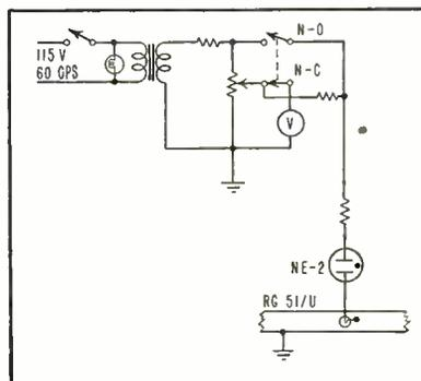
FIG. 1—Magnetron pulsed-power indicator uses extinction point of NE-2 lamp to measure power
