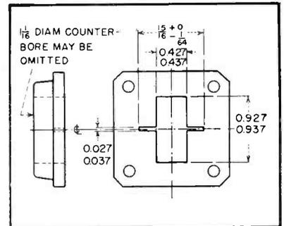
Modifications made in standard UG39U flange for testing lightweight 52U waveguide
