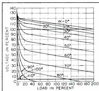
FIG. 3—Regulation curves of a typical ignitron rectifier for steel mill service. Solid sloping lines indicate inherent regulation curves for various angles of delay
