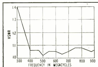
FIG. 2—Graph of vswr over operating range of water load
