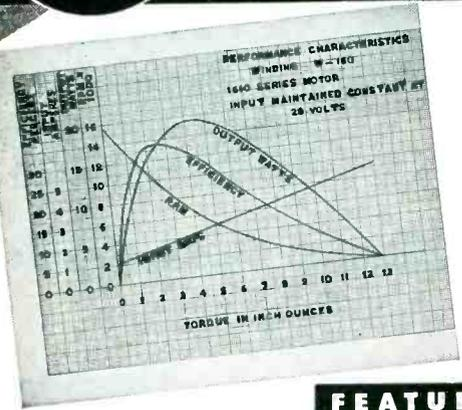
The power output of this precision motor is exceptionally high in proportion to its light weight and small size. Originally developed for numerous aircraft and portable applications, the characteristics of its performance can readily be modified for a variety of new uses.
