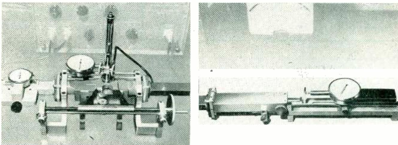
FIG. 2—Left, precision-drive slotted line and attenuator; also x-band precision variable short with finite, calibrated loss, at right
