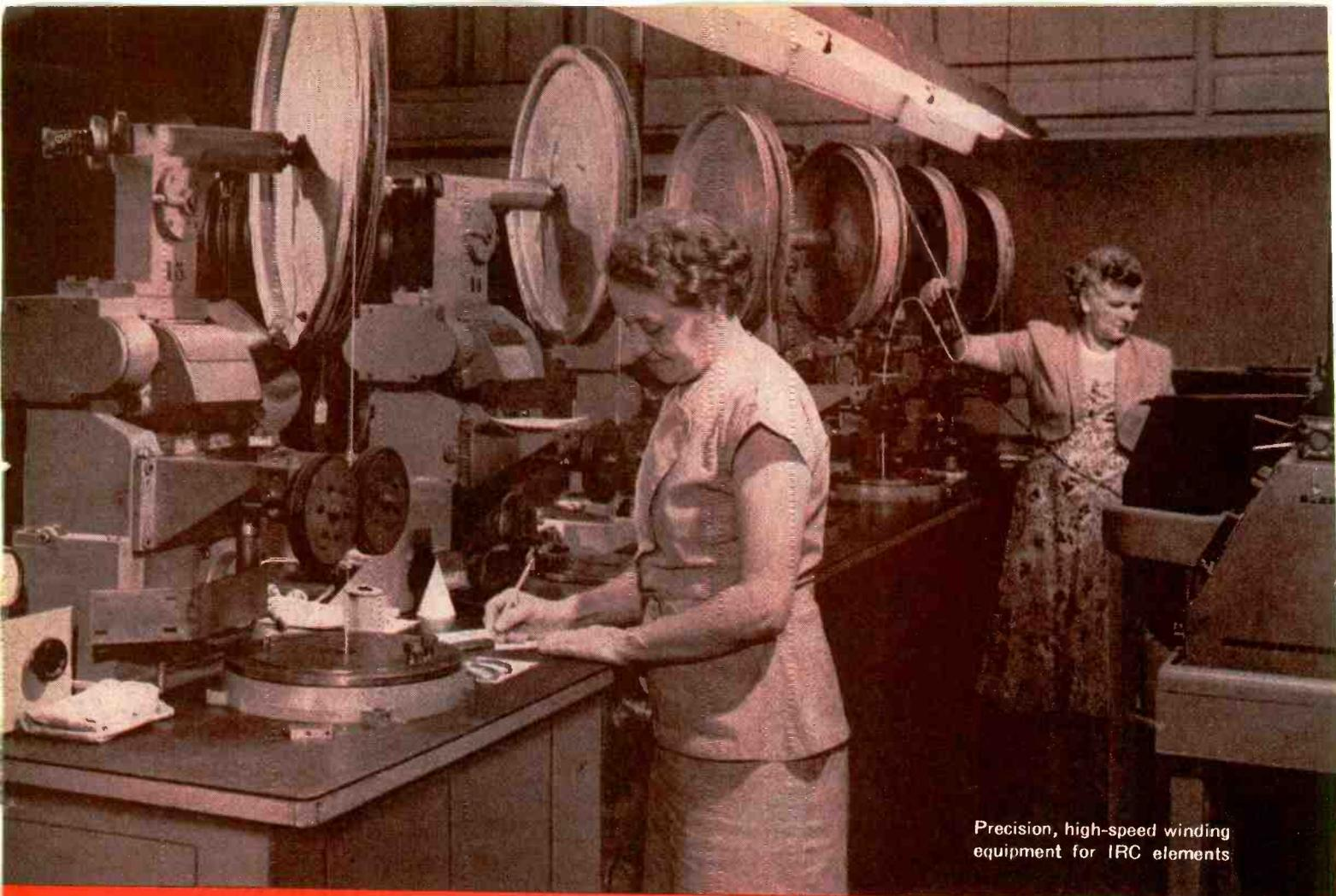
Precision, high-speed winding equipment for IRC elements
