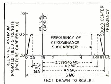
FIG. 1—Idealized picture transmission characteristic, showing relative positions of carriers (item I-D)
