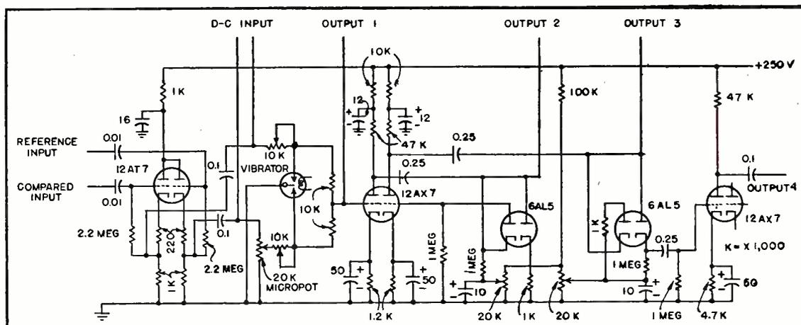
FIG. 4—Modified design comparator is superior to circuit of Fig. 2 but requires special input for d-c signals
