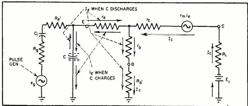
FIG. 8—Basic circuit for one-shot transistor action, where a trigger pulse causes the operating point to move to region III and return to region I without a second triggering pulse
