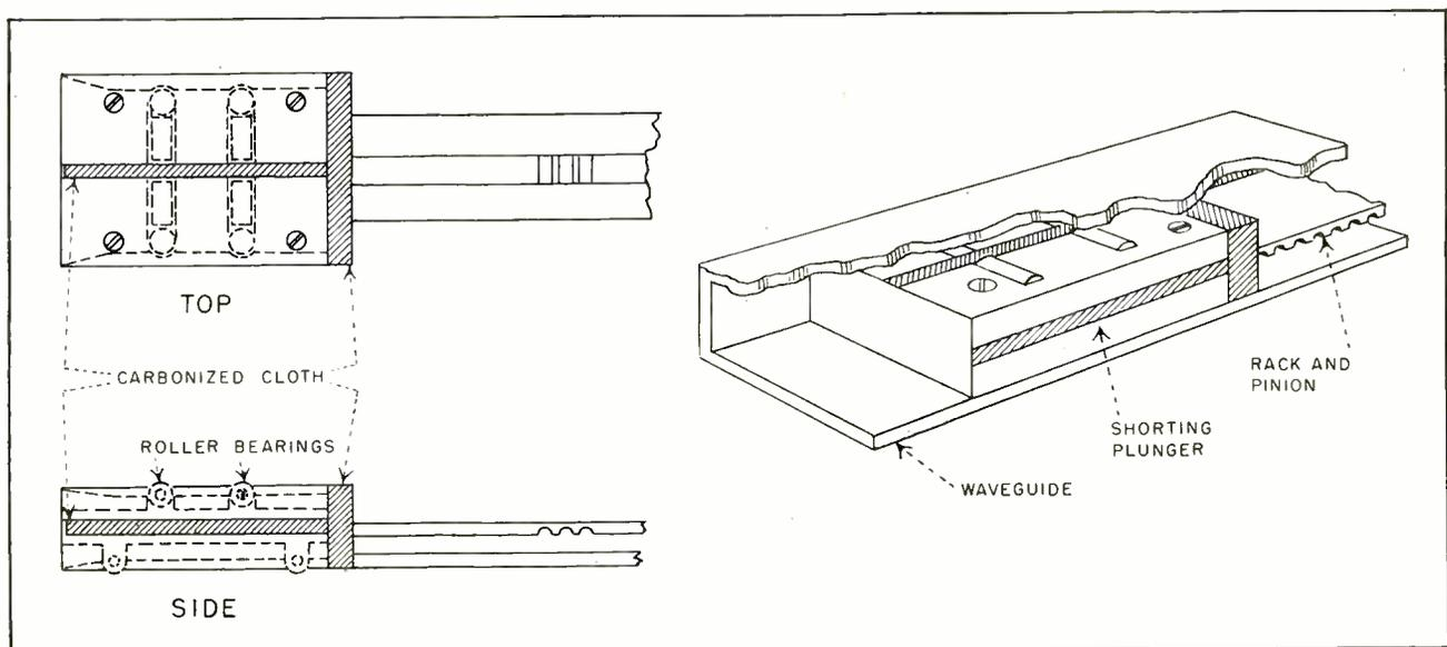
**FIG. 3—Construction of shorting plunger shows how carbonized cloth is used to provide finite, calibrated loss**
