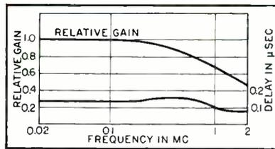
FIG. 3—Phase and amplitude characteristics of feedback-compensated preamplifier described in text
