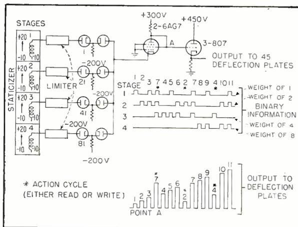
FIG. 8—Binary address digits are converted to weighted currents and summed before being applied to plates
