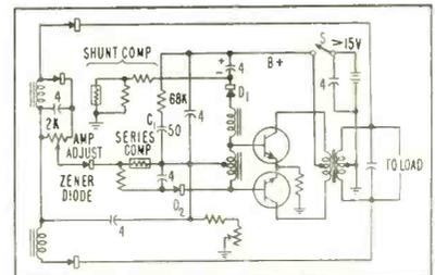
FIG. 1—Audio oscillator circuit uses temperature-compensated Zener diode for stabilization. All transformers windings are on a common core
