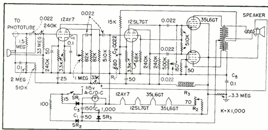
FIG. 1—Circuit of amplifier; d-c to filaments and exciter lamp reduces both light fluctuations and hum
