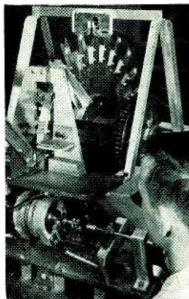
**CAPACITOR PRINTER** applies silver paint to both sides of titanate dielectric pieces. Blank wafers come down chute at left from vibratory feeder
