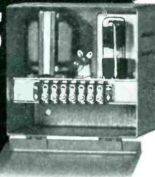
Devtronics engineers have developed three new outstanding basic relay circuits. The sensing elements use activating currents of .1, .01 and .001 micro-amperes with input resistances as high as 500 megohms. Can be furnished with
