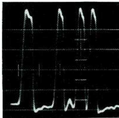
FIG. 3—Same situation as Fig. 2 but with synchroscope gain boosted 30 db so that the second of the 6.67-mc pulses shows more clearly; spurious responses of delay line are here 45 db down
