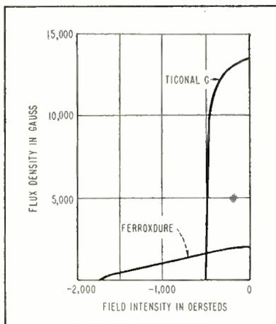
FIG. 3—Demagnetization curve of a ceramic material and a metallic permanent magnet material
