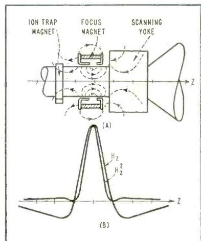
FIG. 1—Permanent-magnet focusing unit (A), and graph of magnetic field intensity (B)
