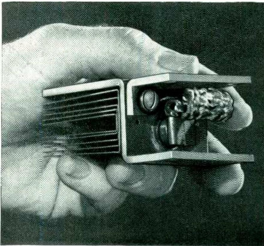
THIS HALF-WAVE GERMANIUM CELL HAS A D-C OUTPUT OF 75 AMPERES AT 26 VOLTS
