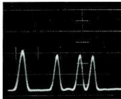
FIG. 2—Timing pulse (left) and four 0.1-microsecond pulses coming out of memory output at 6.67-mc rate, with the second of the four pulses decreased 40 db in input amplitude so that it just barely shows
