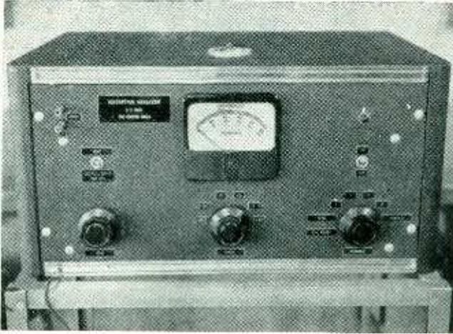
Front control panel of harmonic analyzer has adjustment for input amplitude, meter-range selector and harmonic selector
