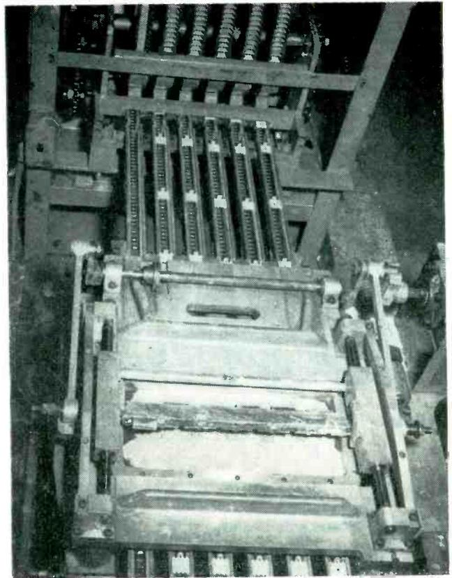
showing some of the six vibratory work feeders that sense the position of orienting notch end tip over any wafers that are upside-down. At right is output end, showing silk-screening.
