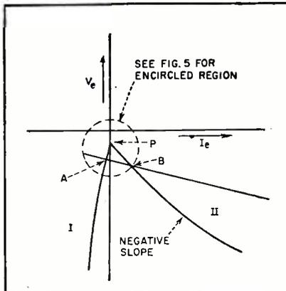
FIG. 4—Emitter characteristic curve in regions I and II. Note negative slope in region II
