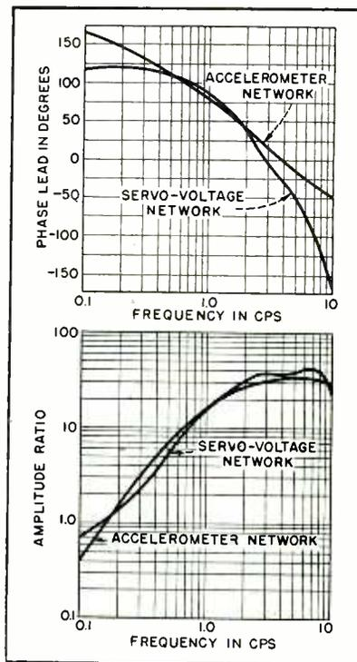
FIG. 6—Comparison of network outputs for disturbances due to turbulence
