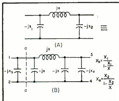
FIG. 2—General pi network (A) can be considered as a balanced pi network with added reactances (B)
