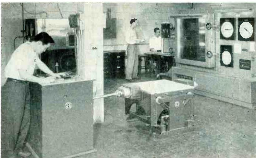
Environmental testing laboratory of the Admiral Corp. in Chicago, Ill includes vibration table in foreground and weather simulating unit at right. The vibration table produces 4,000 vibrations a minute for testing aircraft and shipboard electronic equipment. Climatic-test chambers can subject equipment to a temperature range from  $-100$  to  $185$  F. Relative humidity can be varied from 20 to 98 percent. For testing aircraft equipment, altitudes from sea level to 80,000 feet can be simulated
