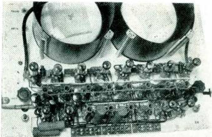
Shields removed from pair of tubes show copper mesh screen held to face of tubes with transparent cellulose tape. Pairs of tubes are rack-mounted (see photograph on opposite page)
