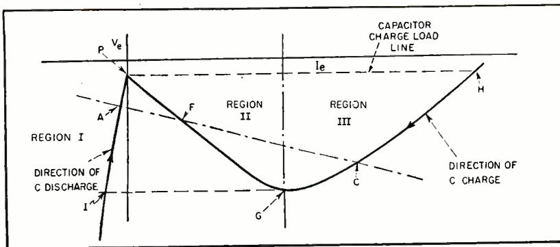
FIG. 9—Emitter characteristic curve for monostable operation of the circuit in Fig. 8. Capacitor  $C$  charges from point  $P$  to  $H$  and to  $G$ , then discharges from point  $I$  back to  $A$
