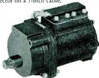
**Electrical Rating:** Rated for operation on 240 volt A.C., two phase, 400 cps. It may also be operated on 208 volt A.C., single phase, 400 cps using a .08 uf capacitor in series with one of the windings.
