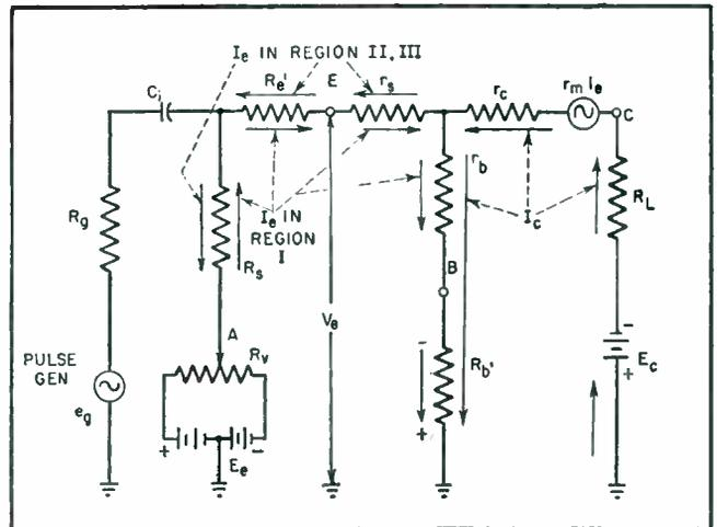
FIG. 2—Basic point-contact switching circuit for bistable operation. Regions are defined in Fig. 7
